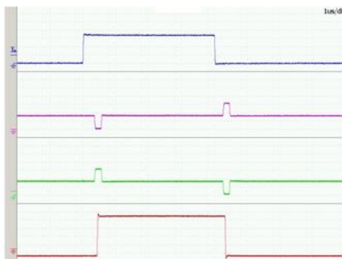
Figure 6. PWM Signal Transmission
